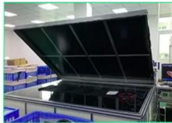
EL testing for foldable solar panel
